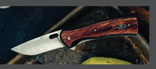
LINER LOCK The liner lock uses a spring-loaded steel liner inside the handle to lock the blade open. The liner can be easily disengaged, allowing for one-handed closing.
